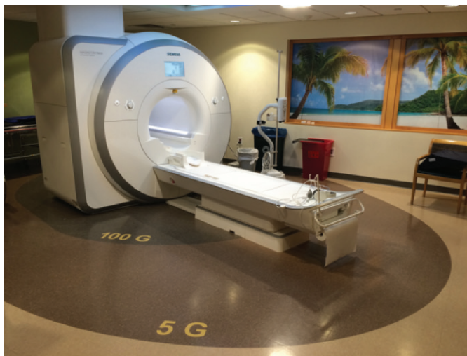
Figure 1. Photograph shows the 5-G line along the floor of one of our MR imaging systems. Newer magnets, such as this 1.5-T unit, use active shielding to bring the 5-G line as close as possible to the bore.
